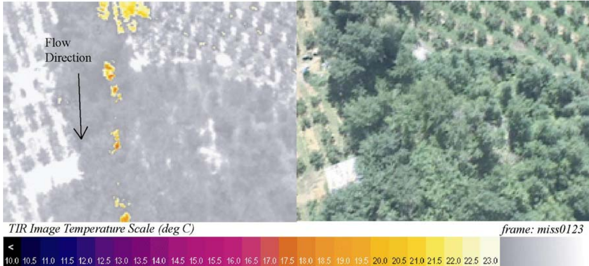
TIR/color video image pair showing an example of Mission Creek (river mile 2.4) and the difficulty in detecting surface water through this reach.
