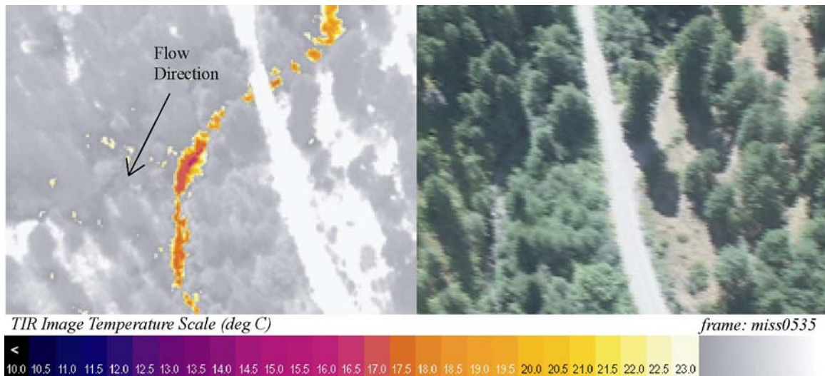
TIR/color video image pair showing an example of the conditions characteristic of the upstream reaches of the Mission Creek survey (river mile 8.6). In the upstream reaches, surface water was clearly visible and had significant thermal contrast from the surrounding vegetation. However, the vegetation precluded detecting small tributaries and other fine scale thermal inflows.
