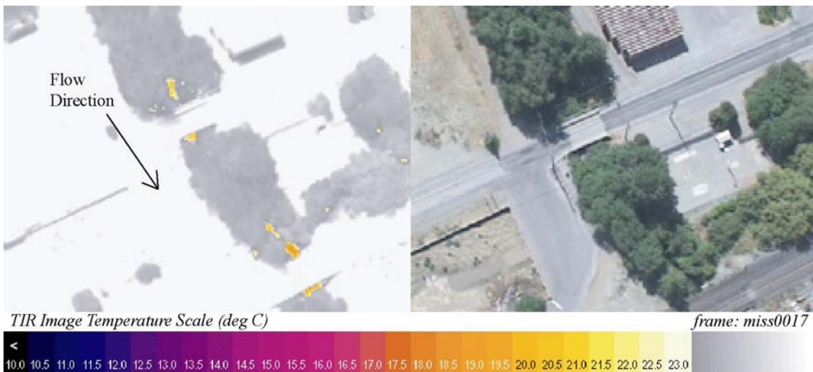
Figure 5 - TIR/color video image showing conditions characteristic of Mission Creek through the town of Cashmere, WA. The confluence of Brender Creek is visible at the very bottom of the image just upstream of the road. In this image, the water surface was visible only near the bridge. In other images, no discernable surface water was visible through the near stream vegetation.
