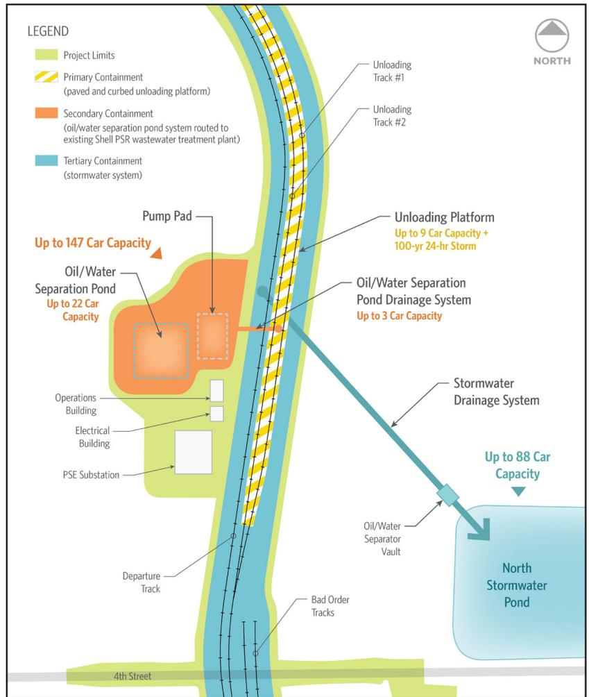
Surface water and spill containment system plan view
