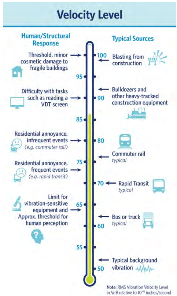
Figure 3.9-2 Typical Vibration Velocity Levels
