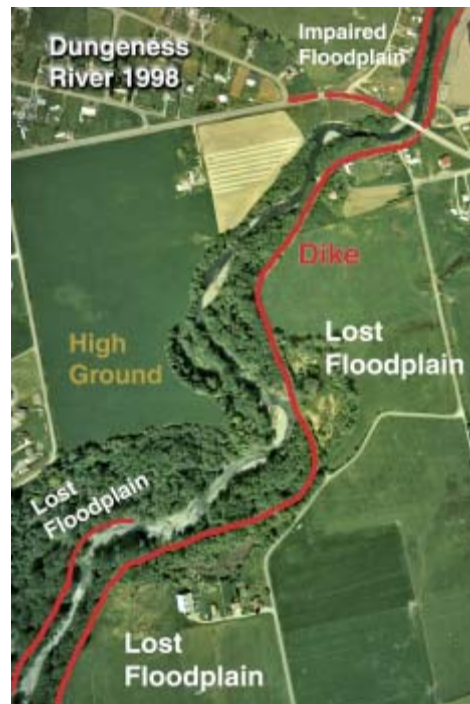
Figure 11. Loss of floodplain access due to diking upstream of Ward Bridge (photo courtesy of Randy Johnson)
