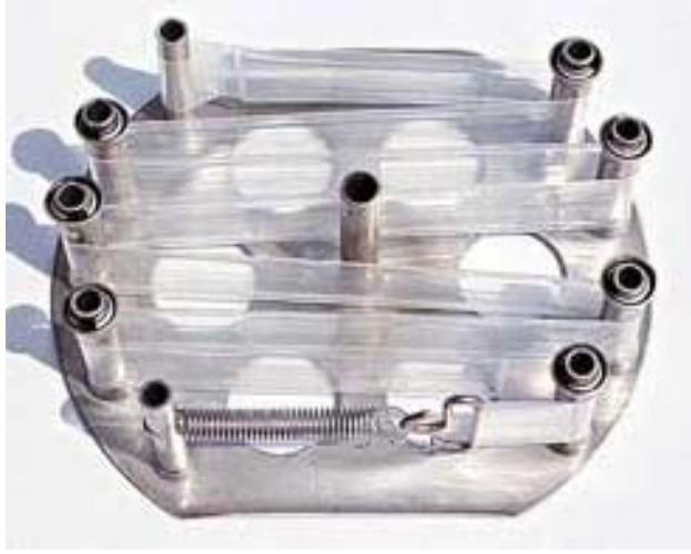
Figure 1. SPMD Membrane on a Spider Carrier
