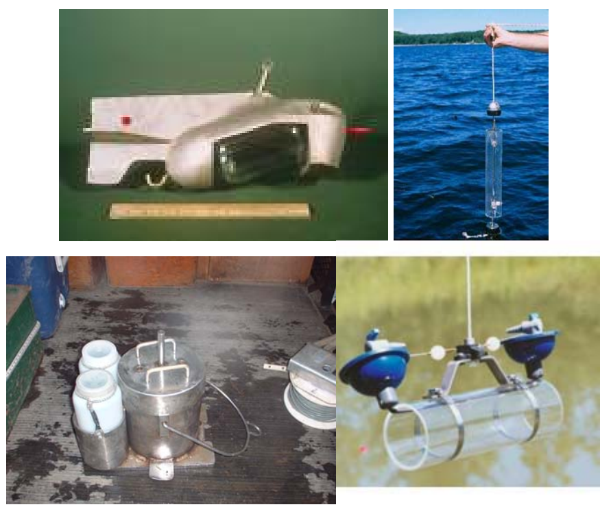
Figure 1. Top: DH-76 integrated sampler with bottle; Kemmerer bottle. Bottom: Weighted bottle and DO bucket for bridges; Van Dorn sampler.
