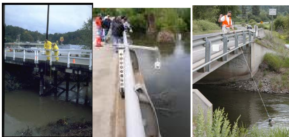
Figure 5. Various methods of collecting water samples from bridges.
