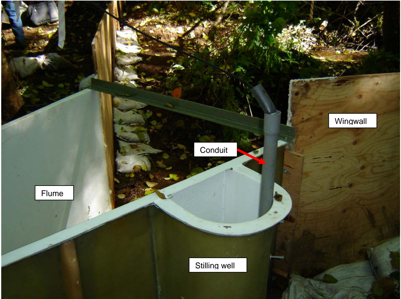
Figure 1. Pressure transducer and conduit in a Type N study stream. Cable ties secure the pressure transducer within the conduit. Holes drilled into the base of the conduit allow water exchange. Bolts secure the conduit to a stilling well and flume.
