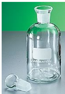
Figure 1. 300mL glass BOD bottle and cap
