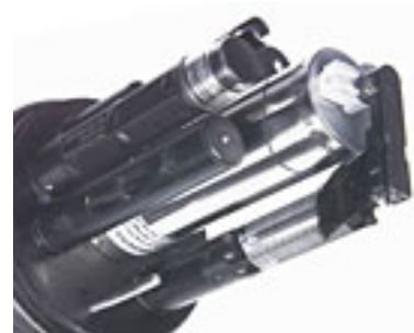
Figure 1. Rhodamine sensor on Hydrolab DataSonde (DS5).
