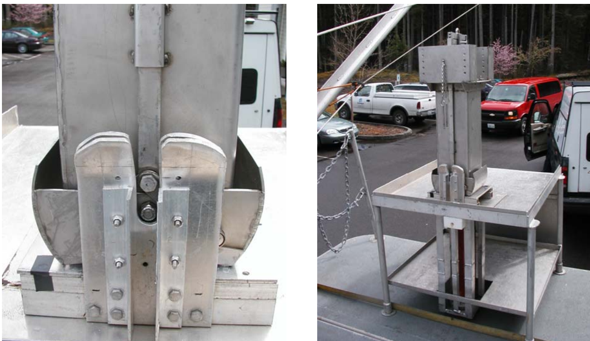
Figure 5. Sediment core placed over the extruding device ready to remove the corer over top of the liner.
