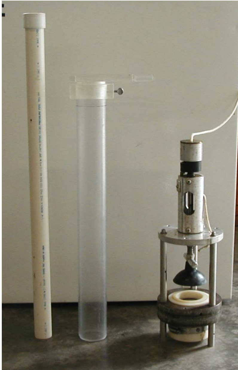
Figure 3. Pictured left to right are extruder, core tube with sectioning apparatus, and sampling housing apparatus.
