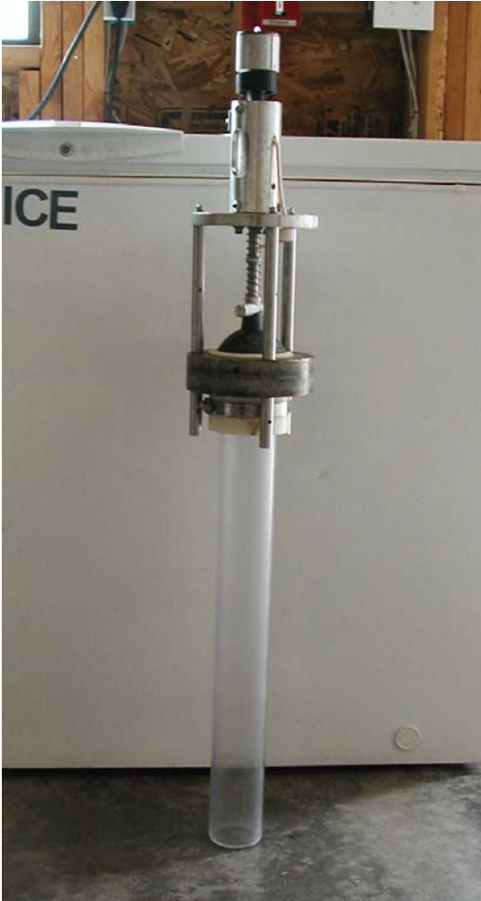
Figure 4. Modified KB corer with suction cup engaged.
