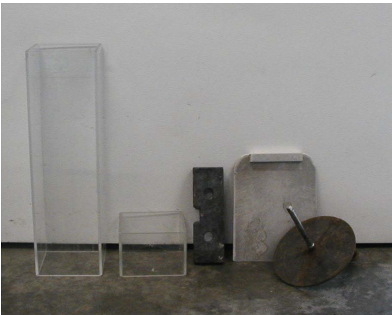
Figure 2: Pictured left to right acrylic liner (50 cm), acrylic liner section, lead weight,, slicing plate, hand crank.
