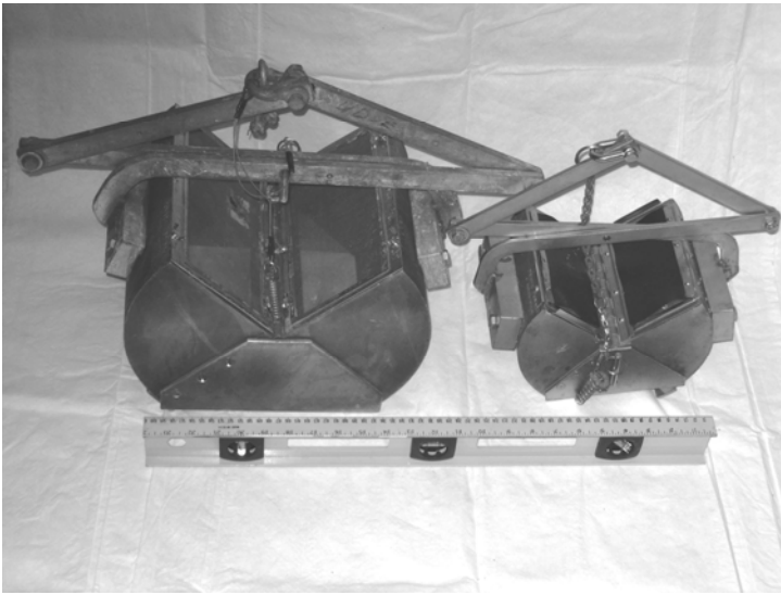
Figure 1. Above: Ponar (left) and Petite Ponar. Right: Tandem Van Veen grabs. Ruler length in both photos is 2 ft.
