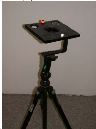
Figure 2: Hemispherical photography tripod and lens mount system.
