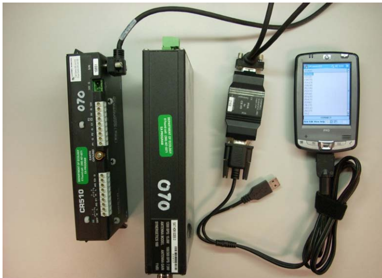
Figure 7: CR510 Datalogger, HDR GOES Radio, CS I/O Adaptor, and PDA with cable connections made for downloading.
