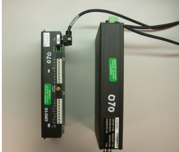
Figure 6: CR510 Datalogger and HDR GOES Radio connected by the "Y" Cable.
