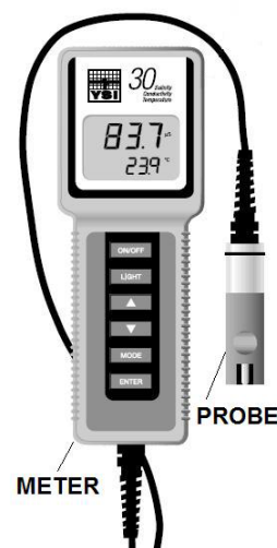
Figure 1. Example of a non-linear Conductivity meter with 4-cell probe.
