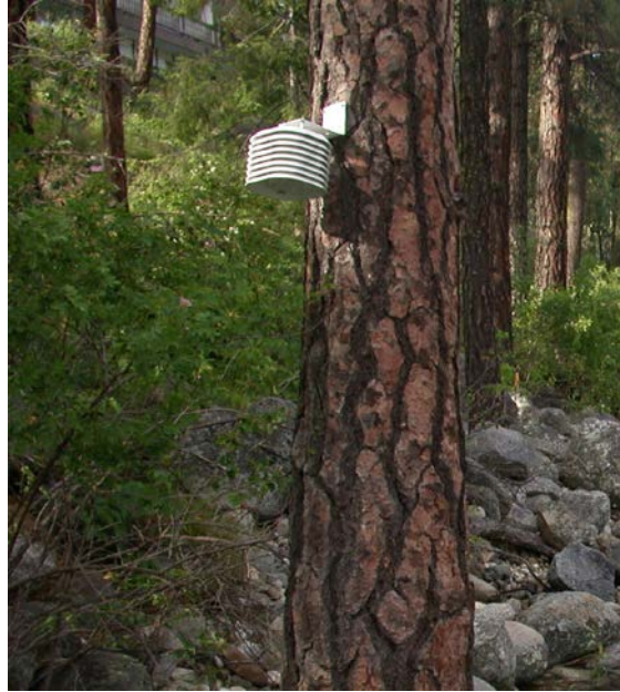
Figure 3: A relative humidity sensor deployed in a solar radiation shield and attached to a tree.
