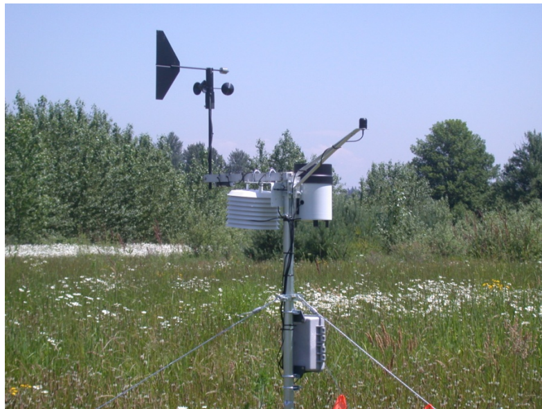
Figure 4: An Onset Hobo weather station deployed near the East Fork Lewis River.
