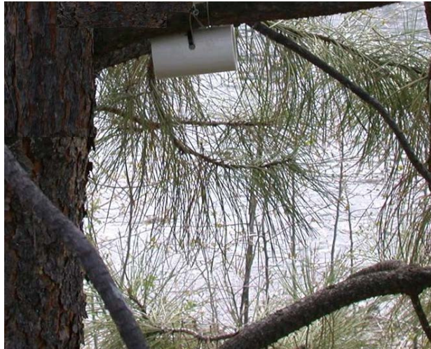
Figure 2: Air thermistor in a white shade device attached to a tree branch.
