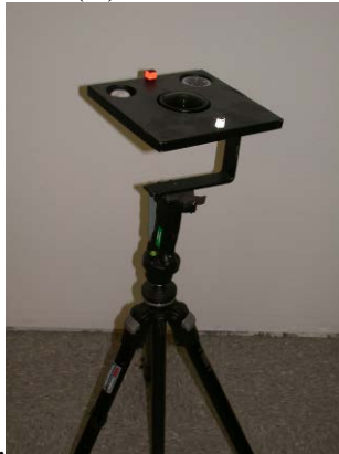
Figure 2: Hemispherical photography tripod and lens mount system.
