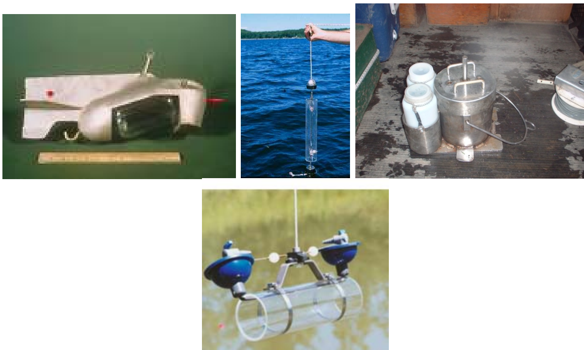
Figure 1. Top: DH-76 integrated sampler with bottle; Kemmerer bottle. Bottom: Weighted bottle and DO bucket for bridges; Van Dorn sampler.
