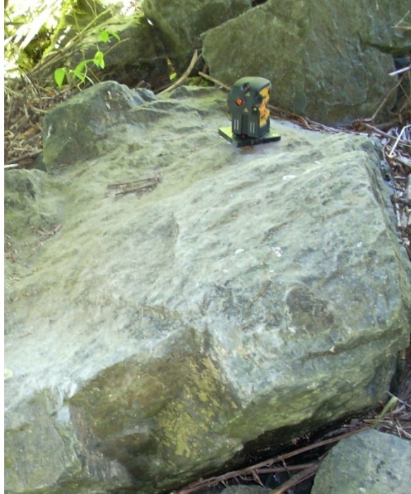
Figure 4 Laser level mounted on laser level pad. (Photo by Washington Dept. of Ecology)
