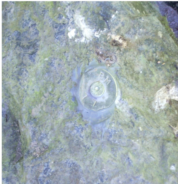
Figure 5 Reference mark placed near laser level is used to confirm elevation of laser level beam. (Photo by Washington Dept. of Ecology)
