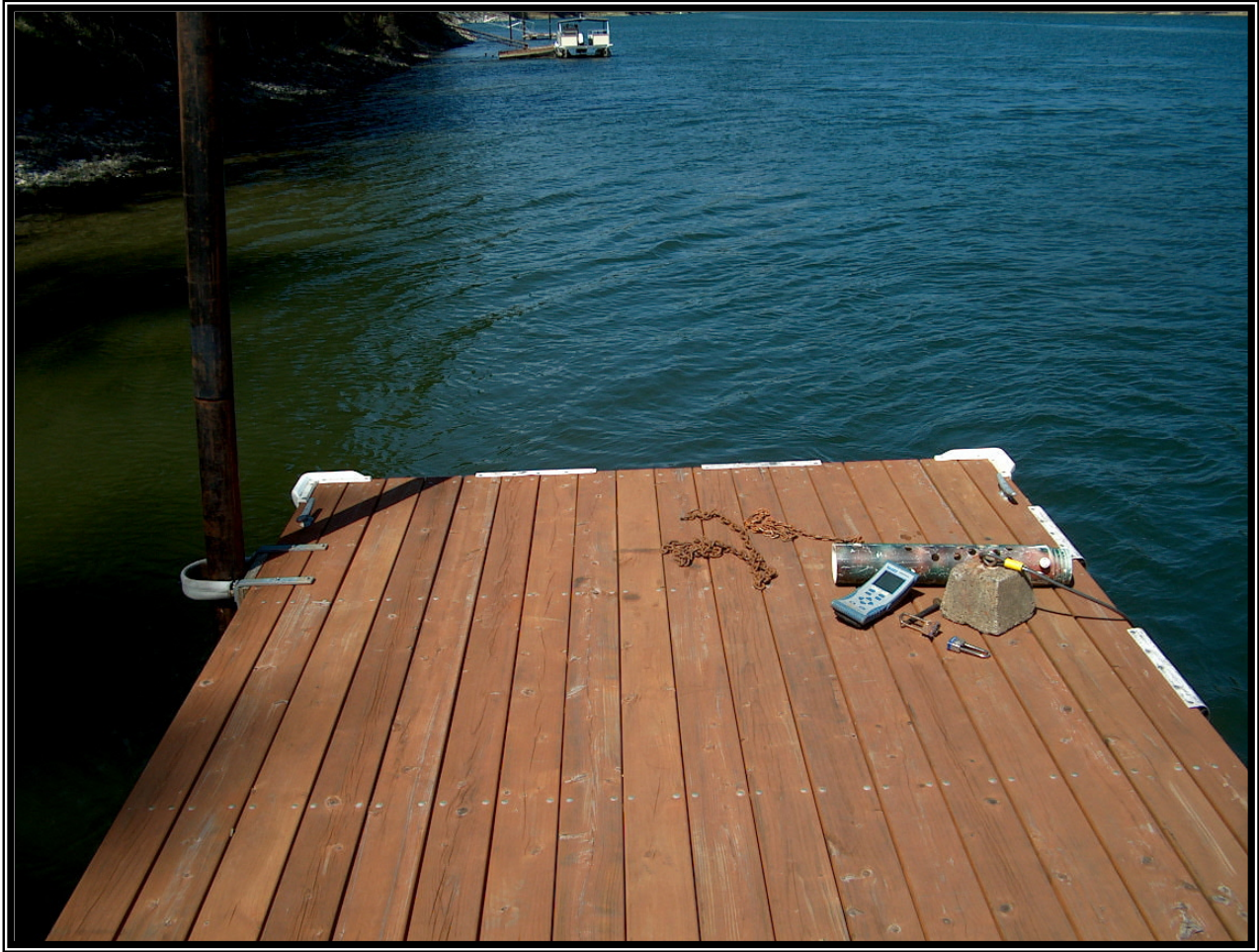
Figure 3. Anchor and PVC housing deployed from a dock for continuous TDG monitoring.
