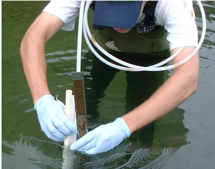
Figure 9 – Using a metric scale and stilling tube to measure relative heads in a tubing piezometer
