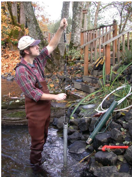
Figure 5 - Deploying a thermistor array into an in-water piezometer
