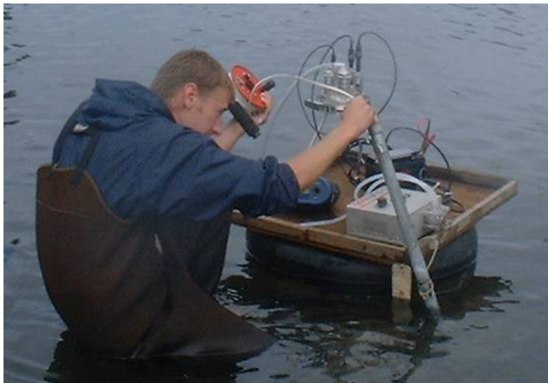
Figure 8 - Using an E-tape to measure the water level in an inclined steel piezometer
