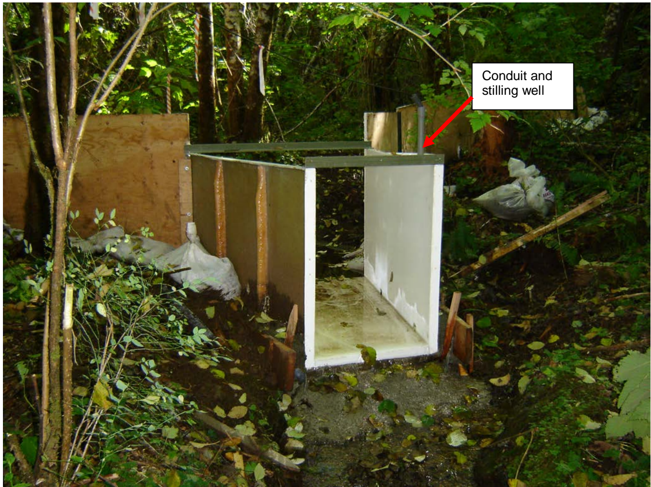
Figure 1. Flume installed in a Type N study stream. A pressure transducer housed within the conduit and stilling well measures stage height.
