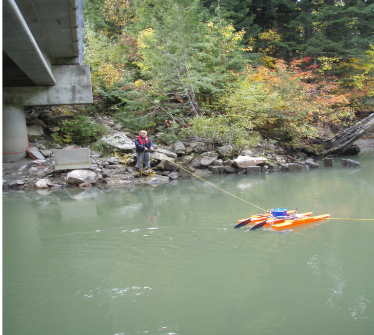
Figure 15. StreamPro raft towed from shore to shore (photo by Washington Department of Ecology).
