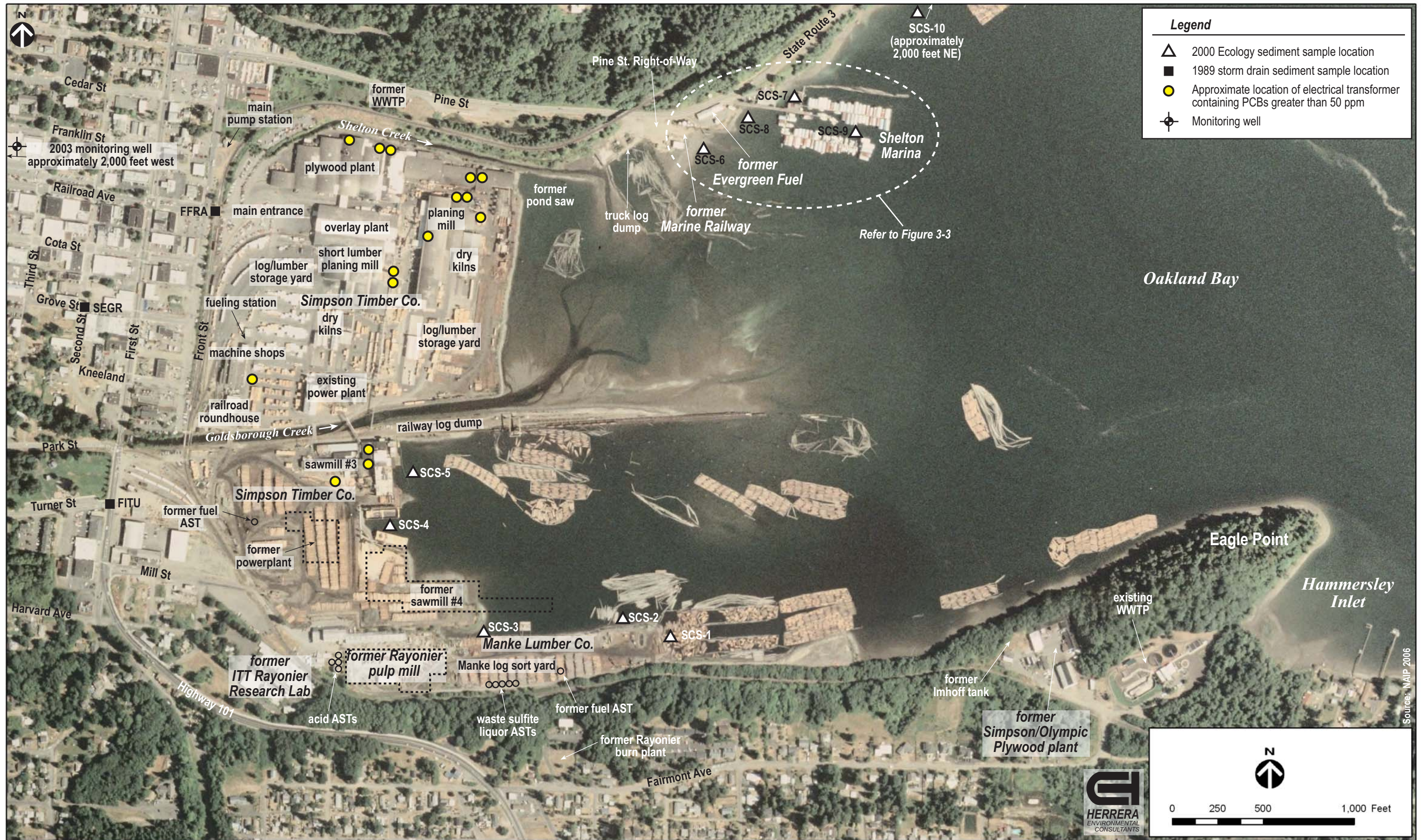
Figure 3-2. Previous investigation sample locations and transformer locations in Shelton Harbor, Shelton, Washington.
