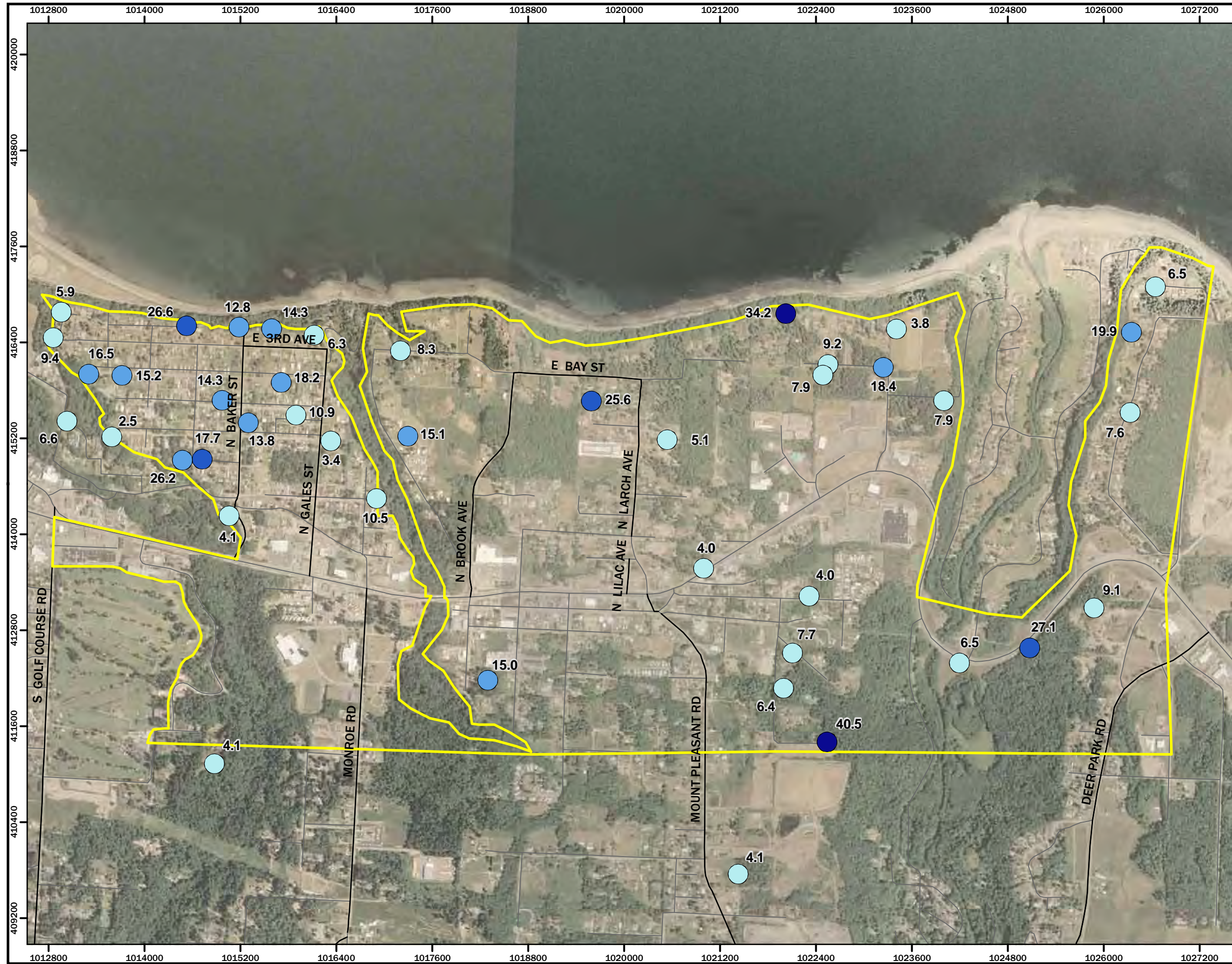
Figure 3-4 TEQ concentrations in Eastern zones. Rayonier Mill Off-Property Soil Dioxin Study Port Angeles, WA.
