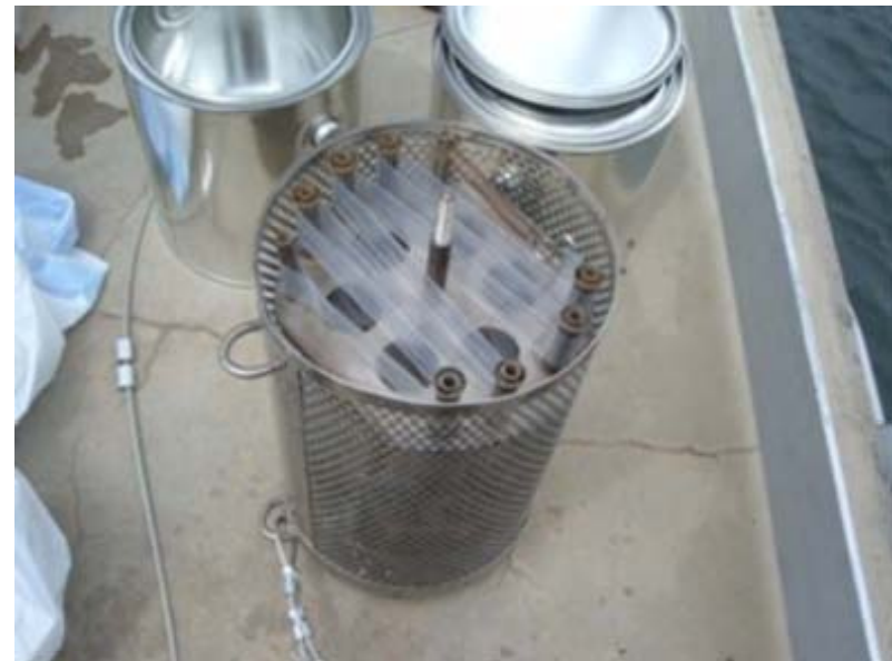
SPMD - Semi-permeable membrane device – passive sampler that allows PBTs to accumulate from water
